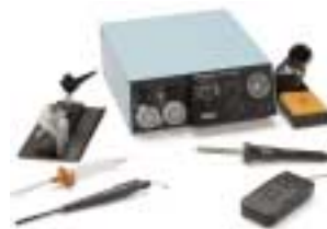
WRS2000 A single channel, analog controlled repair station for use with compressed air or inert gas. The station is supplied with a 100 watt hot air pencil, vacuum pick up and solder paste/adhesive dispenser, all able to be operated simultaneously.
