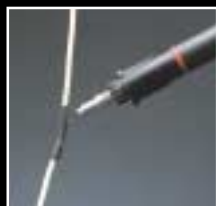
Hot air tip is perfect for heat-shrink applications.
