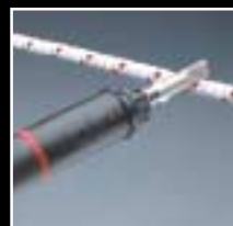
Hot knife tip cuts and seals ends of nylon rope.
