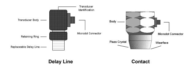
The Transducer is the "business end" of the *PZX-7*. It transmits and receives ultrasonic sound waves that the *PZX-7* uses to calculate the thickness of the material being measured. The transducer connects to the *PZX-7* using a single shielded coaxial cable with microdot connectors.
