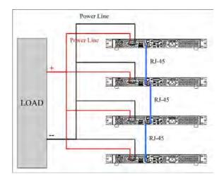
After wiring is complete, configure one XLN3640 / XLN6024 / XLN8018 / XLN10014 as the Master and the other three are Slave A, B and C. After one of the supplies is configured to be the Master, it will start searching for all Slaves that are connected to the Master. Therefore, in order to correctly configure the correctly, user must set up the Slaves <u>before</u> the Master is set.
