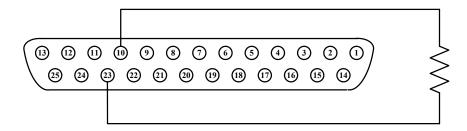
You may access MENU 6-SPECIAL TEST FUNC  $\rightarrow$  2. EXTERNAL CONTROL to choose the input resistance range at [EXTERN PROGRAM =] to [10 V / 10 K] for  $0 - 10 \text{k}\Omega$  and [5 V / 5 K] for  $0 - 5 \text{ k}\Omega$ .
