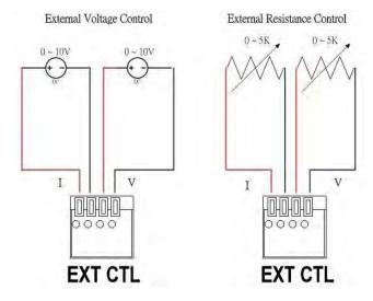
The external voltage control or external resistance control can be set in the "system setting" screen. Since the external control circuit uses a 12bit D/A converter for 0 - 36 V for XLN3640 (or 0 - 60 V for XLN6024 or 0 - 80 V for XLN8018 or 0 - 100 V for XLN10014) output voltage and 0 - 40A for XLN3640
