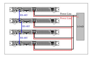
After wiring is complete, configure one of the supplies as the Master and the other three as Slave A, B, and C. After one of the supplies is configured to be the Master, it will start searching for all Slaves that are connected to the Master. To operate correctly, the user must set up the Slaves <u>before</u> the Master.
