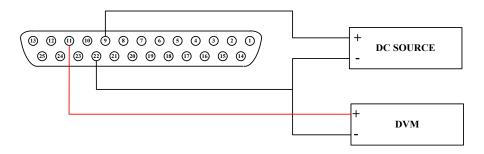
You may access MENU 6-SPECIAL TEST FUNC  $\rightarrow$  2. EXTERNAL CONTROL to choose the voltage monitor output range of Pin 11 at [EXTERN MONITOR=] to [10V] for 0-10 V (as shown in figure below) and [5V] for 0-5V.
