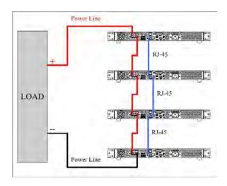
After wiring is complete, configure one supply as the Master and the other three as the Slave A, B, and C. After the power supply is configured as Master, it will start searching for all Slaves that are connected to the Master. Therefore, in order to setup correctly, user must set up the Slaves <u>before</u> the Master is set.
