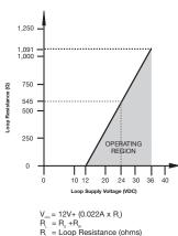
R<sub>s</sub> = Sense Resistance (ohms) R<sub>w</sub> = Wire Resistance (ohms)
