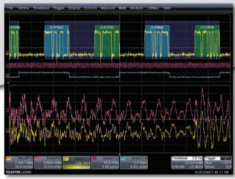
Teledyne LeCroy's unique View Audio feature converts digital audio data into analog waveforms for easy digital audio analysis and debug.
