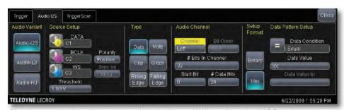
Simultaneously decode up to 4 serial data buses. When using the MSO option on WaveRunner® Xi or WaveSurfer® Xs the digital inputs D0, D1, D2, etc. can be used as the source for a serial data trigger and decode.
