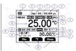
The dot matrix display features a large primary display, smaller secondary displays for channel info or min/max/avg, and helpful annunciators for added measurement data.
