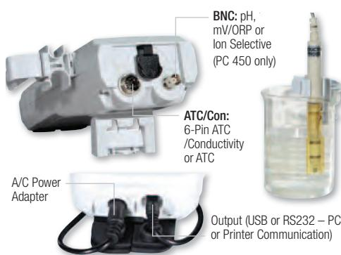
2 mm and 16 mm probes can utilize the Grip-Clip™ to attach one or more sensors to a beaker and to the instrument as needed. The stand can be tended as shown above or used for wall-mounting.
