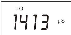
"LO" Battery Condition
