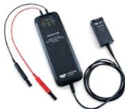
HVDs are rated for wide differential voltage swings - ideal for power electronics circuits.
