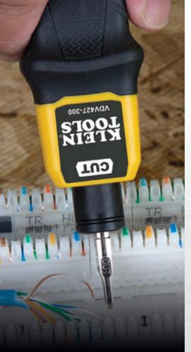
TERMINATE AND CUT WIRES IN ONE STEP
