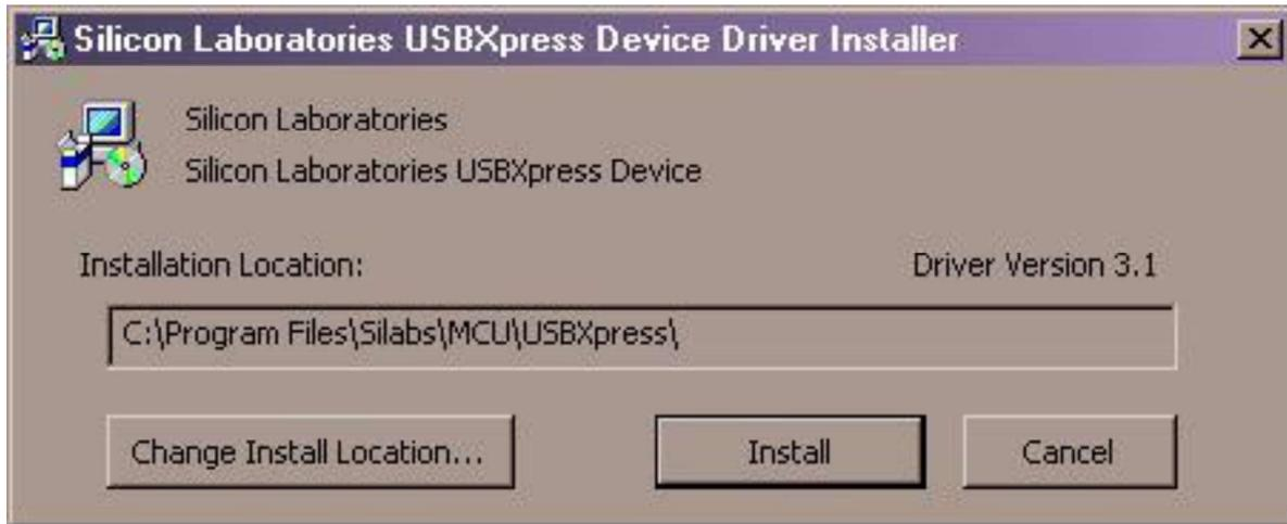
To install the driver manually, plug the VBDL100 into an available USB port on the PC. If this is the first time that the VBDL100 is connected to the particular port on the PC, the following screen will appear:
