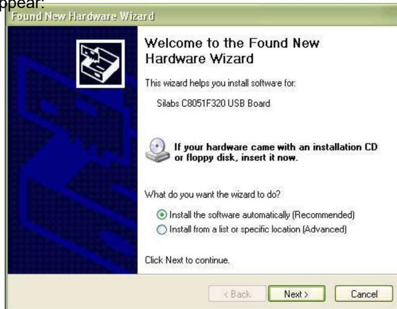
Make sure the program disk is still in the PC CD-ROM drive. Select the 'recommended' installation and follow the on-screen prompts to complete the driver installation. If this is a repeat connection of the VBDL100 to the USB port, the driver installation process will be automatically skipped.
