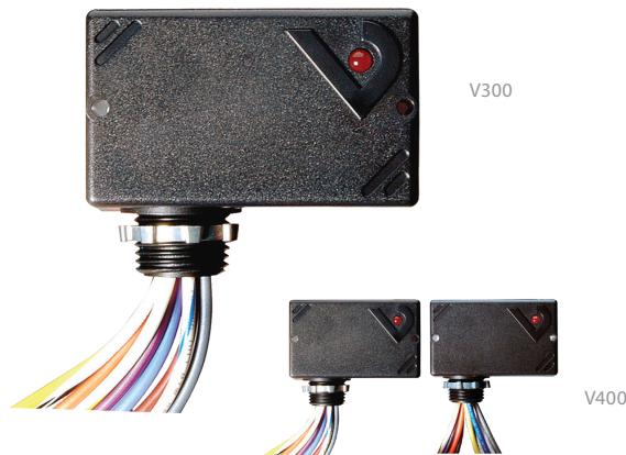
The Victory 300 and 400 Series 10A DPDT pilot duty enclosed relays combine industrial strength and ease of use. The nipple mount enclosure makes installation easy. With no need for a dedicated field enclosure, they are the ideal retrofit devices. One coil input controls the state of two pilot rated contacts for the simultaneous control of two devices or both poles of a single-phase circuit, e.g. motor loads. Field-selectable high and low voltage coil inputs provide on-site versatility.
