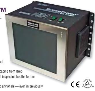
The **UV-400A** features a concentrated-beam reflector designed to assure the highest concentrated UV-A intensity available. It has a peak steady-state UV-A intensity of <u>8,000 µW/cm</u><sup>2</sup> within the lamp's center area, measured at 15 inches (38 cm). The lamp irradiates an area as large as 16" x 10" (41 cm x 25 cm), producing a nominal steady-state UV-A irradiance of not less than <u>2,000 µW/cm</u><sup>2</sup>.
