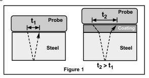
For uncoated materials  $\mathbf{t_1}$  relates directly to material thickness. When a material is coated the propagation time is increased and is shown above as  $\mathbf{t_2}$ .
