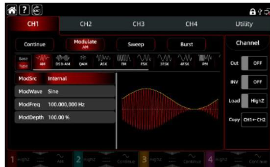
Modulating output (15 types): AM, FM, PM, DSB-AM, ASK, FSK, PSK, 3FSK, 4FSK, B PSK, Q PSK, OSK, SUM, QAM and PWM.
