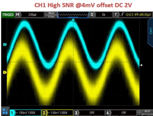
A small signal superimposed with a large DC results in a lower output noise and a higher SNR.
