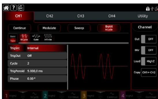
Three pulse string modes: "N cycle", "Infinite" and "Gate". Three trigger sources: "Internal", "External" and "Manual".
