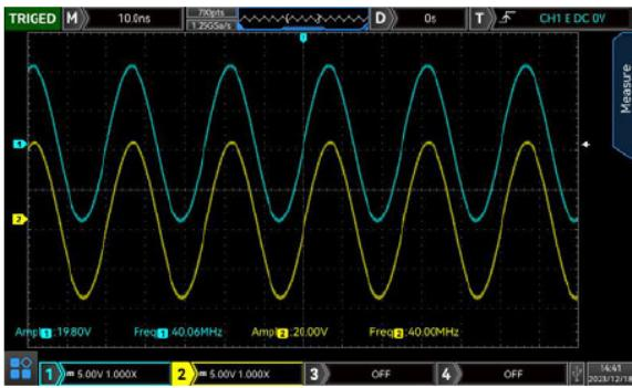
Large output under the high frequency: double channel with full amplitude output of 20 Vpp can be output under the frequency of 40 MHz.
