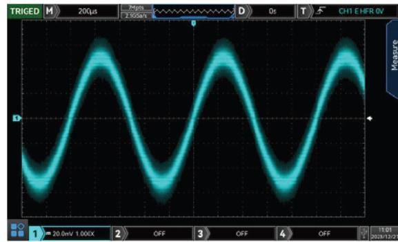
Open the noise superimposition to adjust SNR of signal output.
