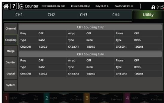
The channel coupling simplifies the operation of double channels. The two channels can use one parameter to control the phase, amplitude or frequency, making it simple to create deviated or proportional signals.
