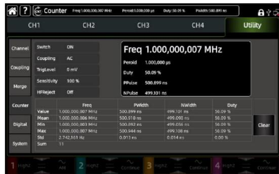
The high precision hardware frequency meter can measure the frequency range of 100 MHz~800 MHz.
