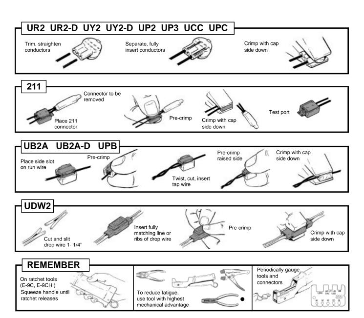
• E9Y tool should **not** be used when crimping three 19 AWG/ .9 mm conductors
