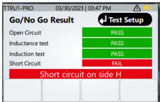
Open circuit ensures continuity through a winding.
