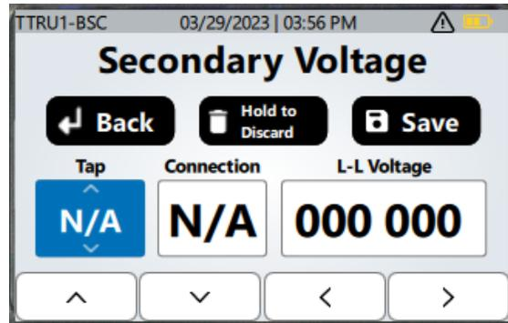
Use the up and down arrows to change the highlighted value. Use the left and right arrows to select a value to change. Press the enter button to return to the previous screen without saving changes. Press and hold the delete button to discard changes. Press the save button to save changes and return to the previous screen.
