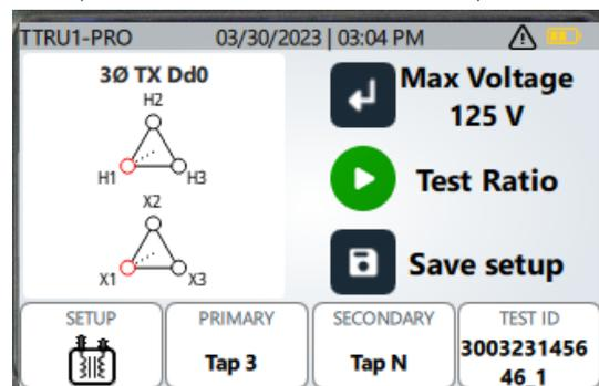
Press the enter key to select the maximum test voltage from the following options: 1 V, 4 V, 8V, 16 V, 32 V, 50 V, 80 V, 125 V, 160 V, 200 V, or 250 V. Voltages above 50 V will use the step up method of ratio testing.
