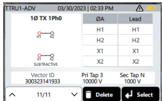
Use the up and down buttons to change the displayed vector. Press the enter button to select the displayed vector. The instrument will return to the test setup screen with the vector selected.
