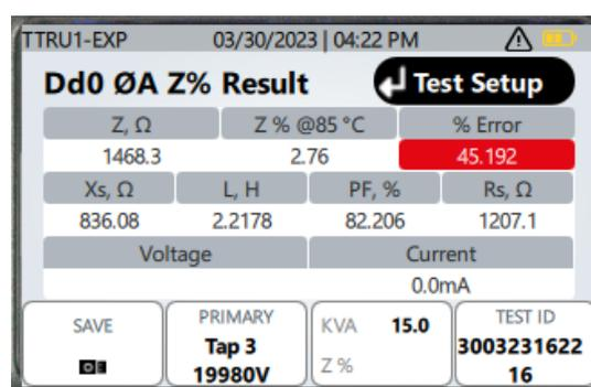
Click and hold the enter button for three seconds to view additional test information, including measured impedance, reactance, inductance, power factor, and AC resistance, and test voltage and current.
