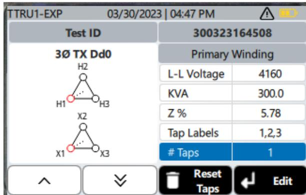
Press the up and down arrows to select a nameplate field to edit.
