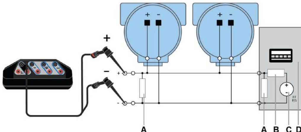
For small fieldbus segments, the power conditioner and terminators can be contained in a single wiring block.
