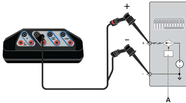
The Trex unit is connected to an analog output and is measuring current from the mA terminals. You can connect the Trex unit at various points on the current loop, including a junction box, device connection point, etc.
