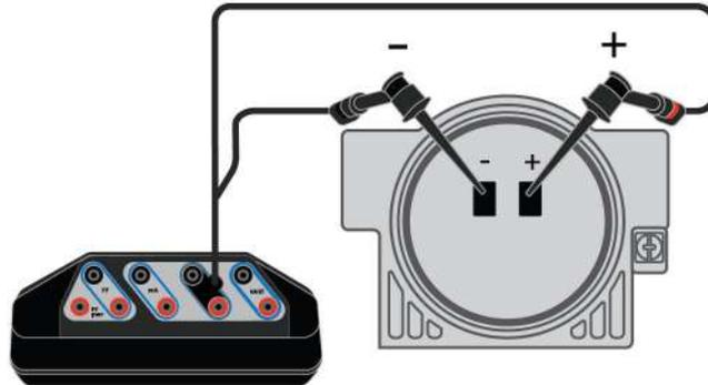
The Trex unit measures both voltage and current from the HART + pwr terminals.
