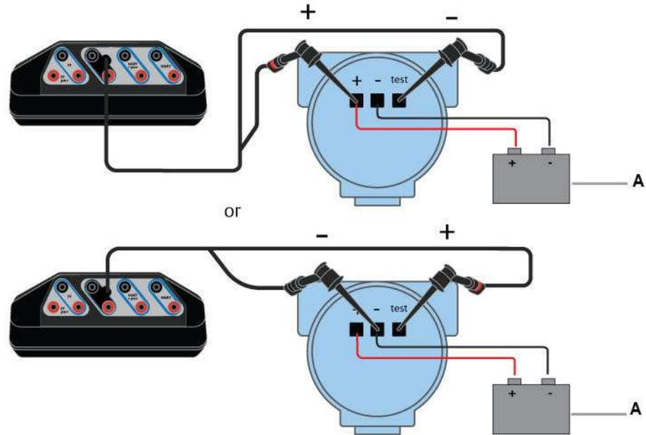
The Trex unit measures current from the mA terminals on an externally-powered loop without breaking the loop and connecting the ammeter (mA terminals) in-series.
