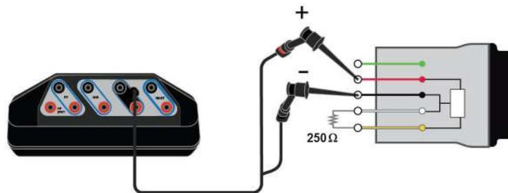
Connect the lead set to the red and black wires.
