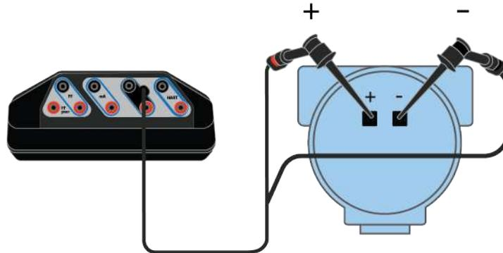
The Trex unit measures both voltage and current from the HART + pwr terminals. An internal 167 Ohm resistor is used when the Trex unit powers the device.
