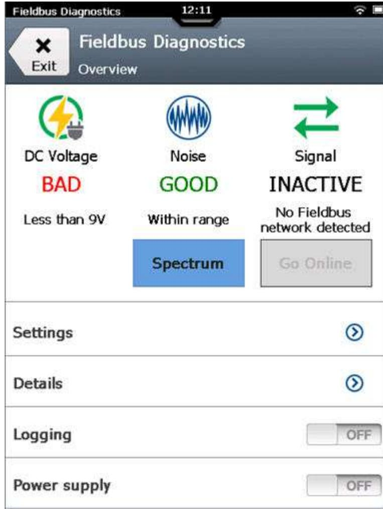
Figure 5-2: Fieldbus Diagnostics Overview screen while taking measurements
