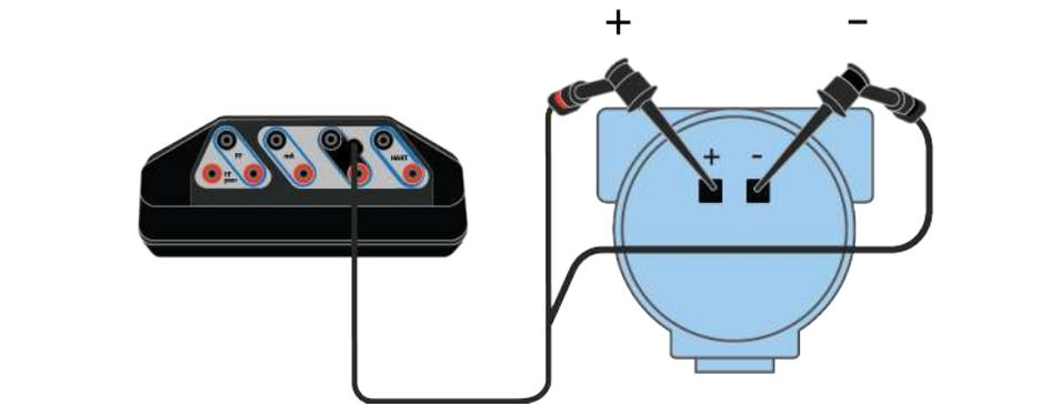
**Figure 3-30: Power a HART positioner**
