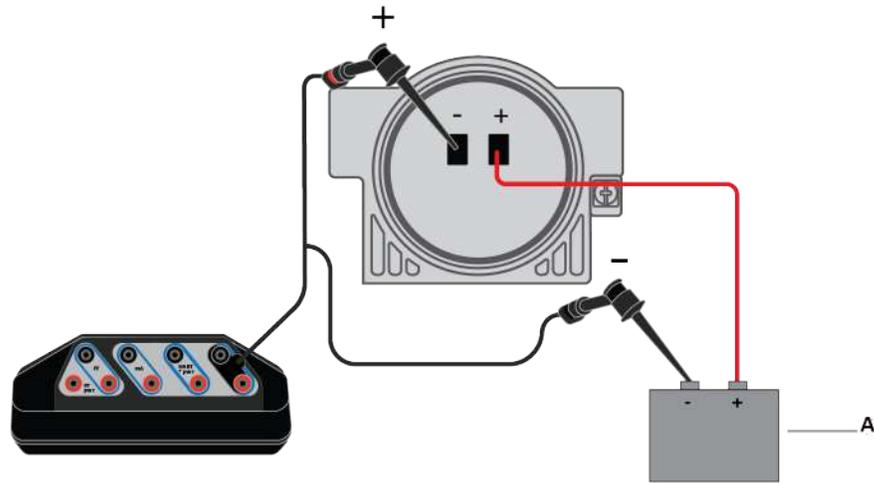
The Trex unit controls current from the HART terminals.
