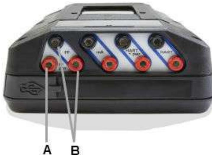
A. FF pwr terminal provides power, power conditioning, and two terminators to one FOUNDATION fieldbus device. Use the FOUNDATION fieldbus Power Plug to connect this terminal to the red FF terminal.
