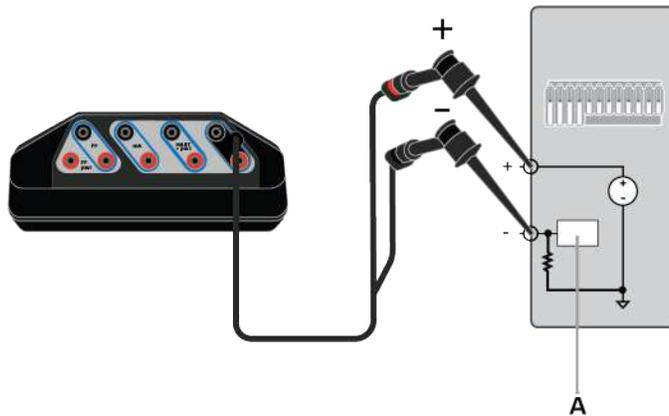
The Trex unit controls current from the HART terminals, which simulates a transmitter. The Trex unit controls current the same way as a transmitter controls current. The Trex unit is connected to the analog input (AI) channel.
