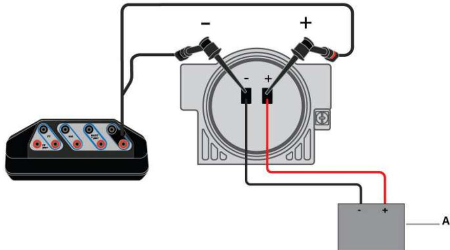
The Trex unit measures voltage from the HART terminals. Voltage measurements can be taken at various points to identify voltage drops along the loop.
