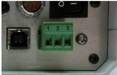
Figure 1: Relay screw-terminal header
