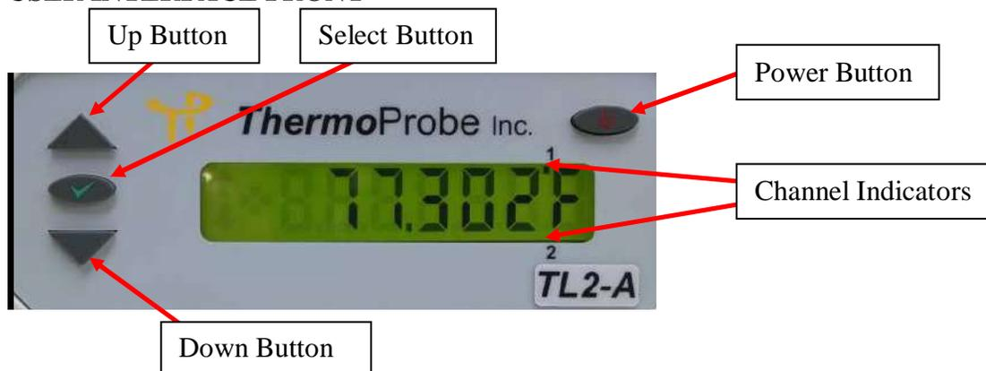
**Power Button (AC Unit)** – Use the power button to save your settings (temperature units, display decimals, zero adjustments, relay settings, etc.), and to place the TL2-A in ‘Standby’ mode. If you remove AC the power without putting the TL2-A in Standby mode, the user settings will revert to the previous settings.
