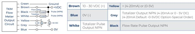
Black Wire can be Changed for Flow Total Limit Output or Unit Volume Pulse Output
