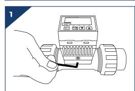
Using an allen key loosen the 2 screws located on either side of the display.
