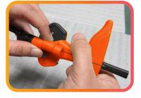
**Step 4.** Pull the cables and tool in the opposite directions to strip the cable.
