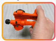
**Step 2.** Insert the fiber optic cable.
