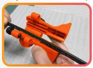
**Step 3.** Close the tool making sure the plunger is in the locked position.
