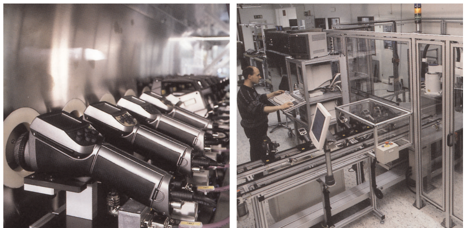
Figure 28.5 LEFT: Testing of infrared cameras in the climatic chamber; RIGHT: Robot used for camera testing and calibration
