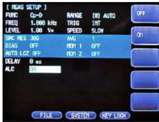
Automatic Level Control Ideal for Measuring Components With Voltage Requirements
