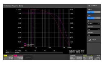
The oscilloscope can control the built-in waveform generator or a stand-alone Teledyne Test Tool generator, to scan the amplitude and phase-frequency response of the DUT, and display the data as a Bode Plot. This makes it possible to replace expensive network analyzers in some applications.
