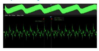
Using hardware-based Zoom technique and record length of up to 200 Mpts, users can select a slower timebase without compromising the sample rate, and then quickly zoom in to focus on the area of interest.
