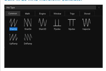
The built-in waveform generator can output waveforms with up to 25 MHz frequency and ±3 V amplitude. Six basic waveforms together with multiple types of predefined waveforms and as user-defined arbitrary waveforms are supported. (Optional USB 50 MHz AWG module: T3DSO-FGMOD)
