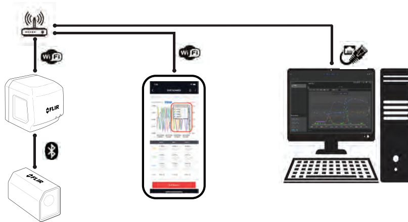
Figure 8.2 Block diagram of a system controlled by a Windows PC. The GW65 Gateway communicates with the SV87 Sensor using Bluetooth and with the smart phone through a Wi-Fi router. The PC is shown communicating with the network using a direct Ethernet connection.
