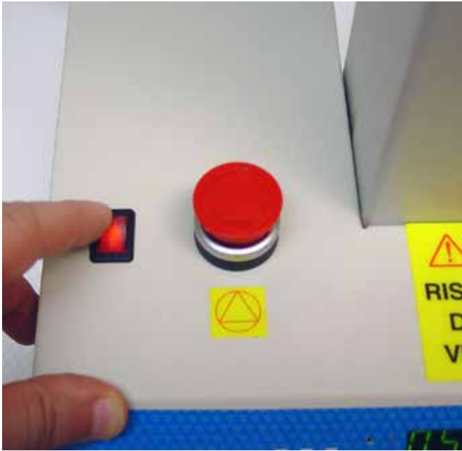
The ON/OFF switch is a 2-way switch. The switch is lighted when power is ON.
