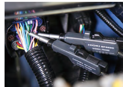
Undamaged wires for easy and safe measurement
