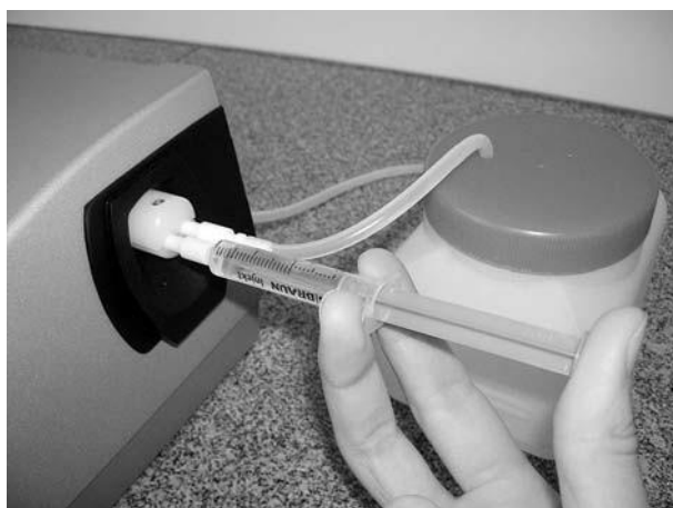
Fig. 12 - 1 Filling sample using the plastic syringe
