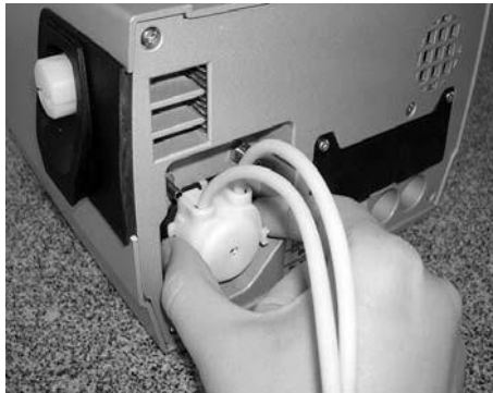
Fig. 7 - 2 Removing the pump cassette
