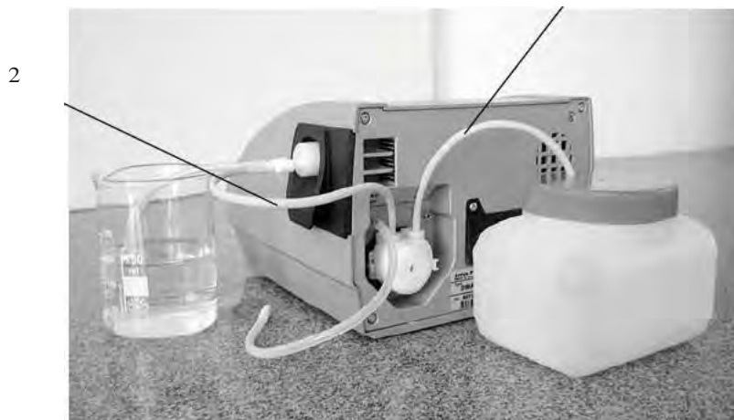
Fig. 7- 3 Filling with the peristaltic pump
