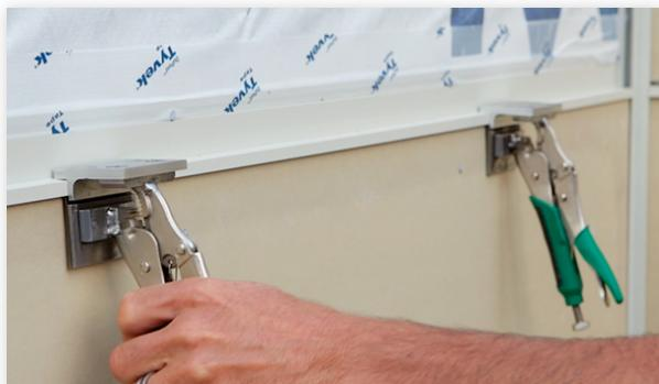
To adjust siding-to-flashing gap, simply remove or add the included spacer plates. Sliding the spacer plates forward adjusts for the siding thickness, while the tension knob adjusts for flashing thickness.
