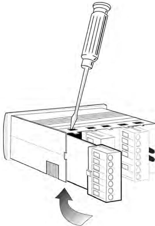
**Figure 4. Removing Option Module**
