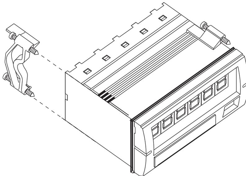
Figure 3. Panel Mounting Clips
