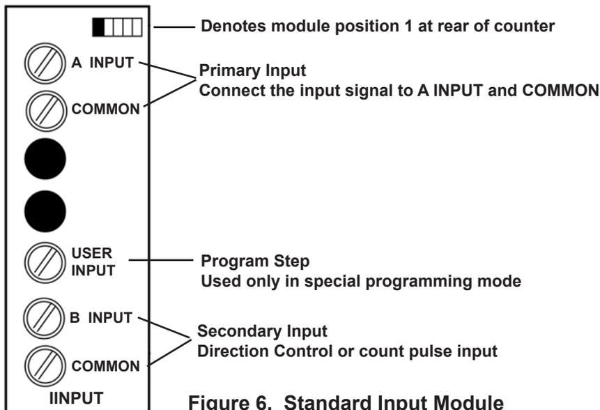
Figure 6. Standard Input Module
