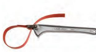
The Klein Tools 18-Inch Grip-It Strap Wrench is completely adjustable for tight-quarters tasks on polished, PVC and glass pipes, fittings, filters, conduit and shafts. The strap is urethane-coated to resist scratching or damaging surfaces and is attached to a lightweight I-beam handle. Also available in 6-Inch and 12-Inch lengths (Cat. No. S6H and S12H).
