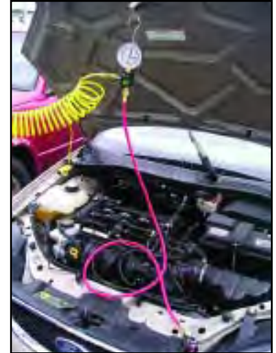
NITROKIT : includes the NITROKIT with a nitrogen regulator.
