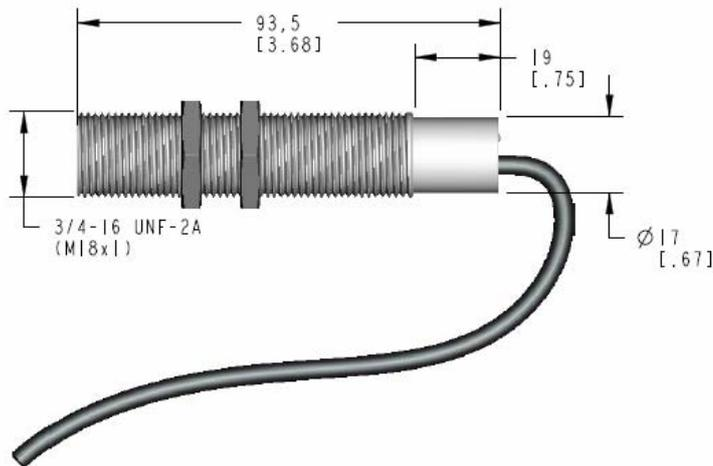
Figure 3: Dimensions of sensor
