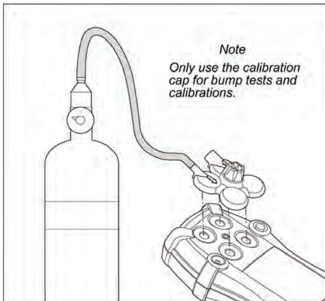
Figure 11. Connecting the Gas Cylinder to the Detector
