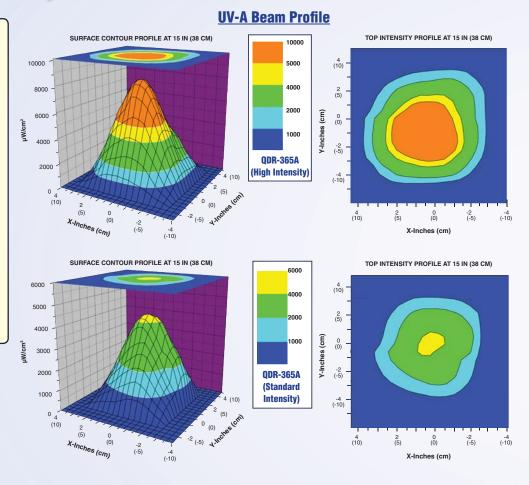
Typical wavelength output profile of QUADRAN™ 365 Series lamps with and without black light filter.
