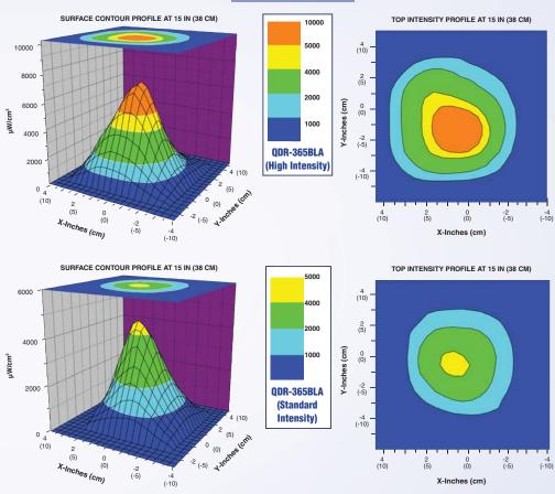
The QDR-365BLA is equipped with a faceplate with integral black light filters that reduce the output of wavelengths longer than 400 nm. When in the high intensity mode, the lamp provides a nominal steady-state UV-A intensity of 7,000 µW/cm² at 15 inches (38 cm).
