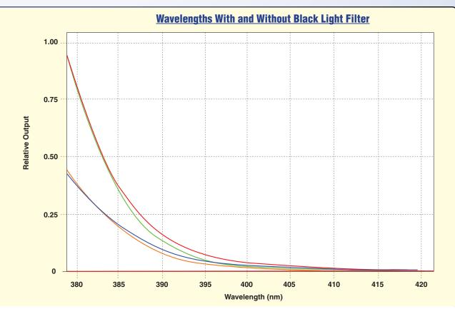
As the wavelength of the QUADRAN™ 365 moves into the visible light range, the black light filters significantly reduce the output of the lamp at 400 nm.
