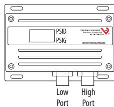
4. Connect the other ends of the tubing to a pipe or duct, across the pump, filter, or other pressure differential.
