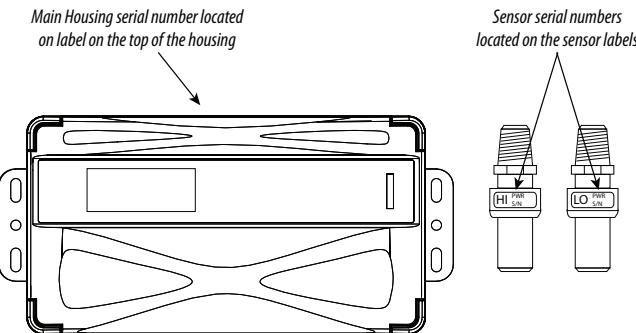
5. Run wires from the remote pressure sensor cables and connect to the pair of 4-terminal blocks at the right side of the board. To maintain the correct calibration, it is important not to confuse the high side and the low side. To assist, the sensors are labeled, "HI" and "LO."
