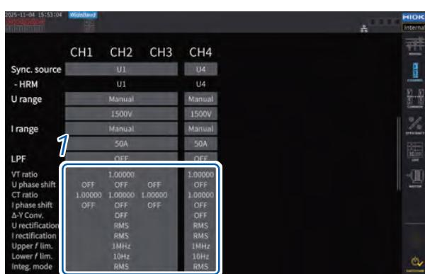
1 Tap the channel detail display area for the channel you wish to configure to open the settings window.
