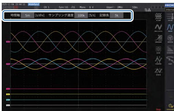
Tap each box and then rotate the X rotary knob to set each setting items.
