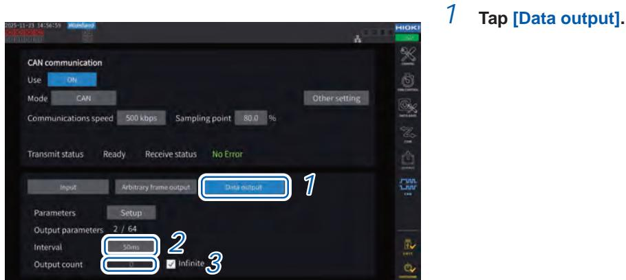
2 Tap the **[Interval]** box and select a CAN-signal-outputting interval from the list.
