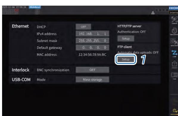
1 Tap the **[Setup]** box under **[FTP client]** to open the setting window.
