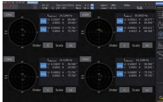
The 4-vector-diagram display illustrates four graphs of each selected wiring configuration.
