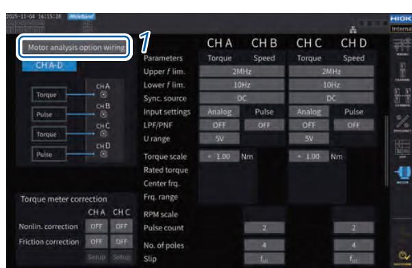
1 Tap **[Motor analysis option wiring]** to open the settings window.
