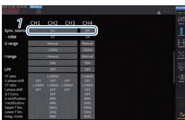
1 Tap the **[Sync. source]** box of the wiring configuration you wish to set to open the setting window.
