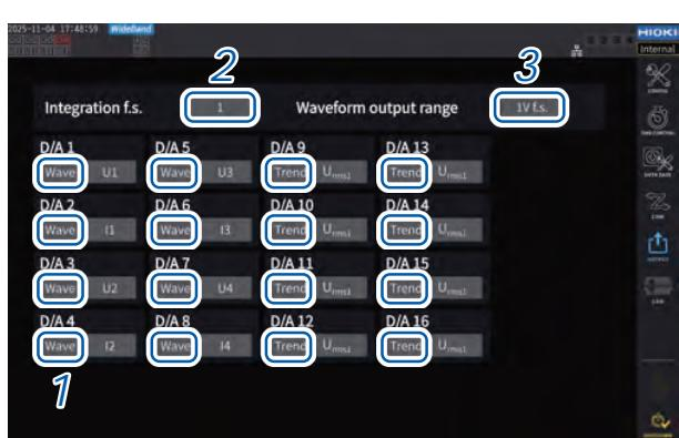
1 Choose between the two output types: **[Trend]** and **[Wave]** for each channel.
