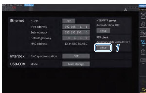
1 Tap the **[Setup]** box under **[FTP client]** to open the setting window.
