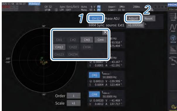
1 Select the channel for which you wish to perform phase angle zero adjustment using the channel selection window.
