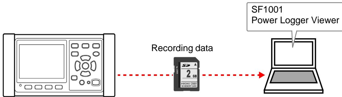
To access data, either load it from the SD memory card on which it was saved using a computer with an SD memory card reader, or use a USB cable to copy data from the SD memory card or internal memory to the computer.
