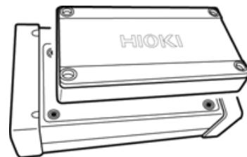
**7** Install the battery case onto the instrument using the four dedicated screws (M3×25 mm) that come with Model PW9002 Battery Set.
