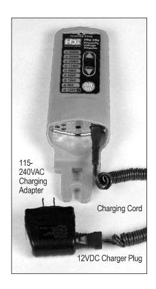
If the instrument will not turn on, try charging it for fifteen minutes. The battery may be drained down too far to be able to power on. If it still will not turn on then the battery may need to be replaced. For battery replacement contact HD Electric to order a replacement battery.
