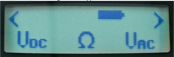
Connect the Pro50<sup>™</sup> to the zone or item you wish to test. Press F1 for DC Voltage, F2 for resistance ohms, or F3 for AC Voltage. The Pro50<sup>™</sup> has auto-range capability, meaning that the expected range is not required to be entered into the Pro50<sup>™</sup>.
