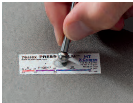
Stainless Steel Burnishing Tool ensures consistency
