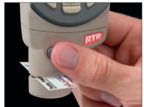
Align probe arrows with tape positioning dots
