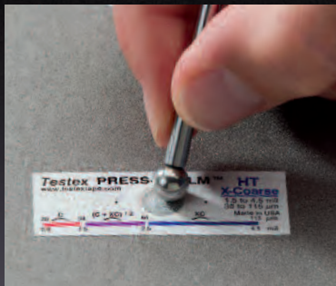
For use with Testex™ Press-O-Film™ Replica Tape
