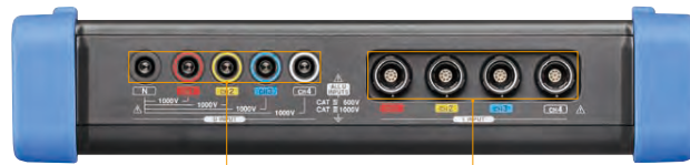
Voltage input terminals (4 channels)
