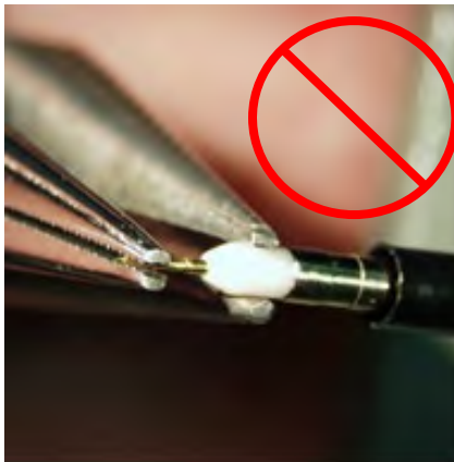
Do not apply pliers to the plastic insulator.
