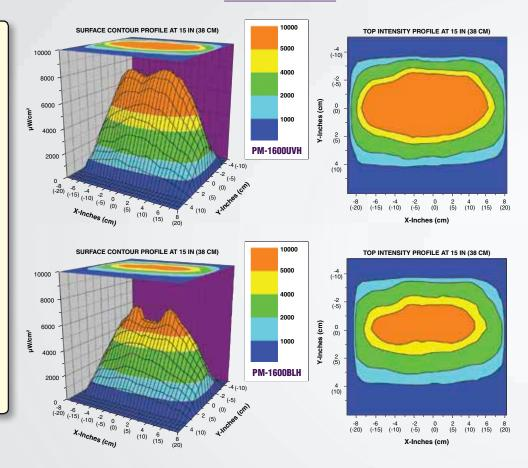
Typical wavelength output profile of PowerMAX<sup>™</sup> 365 Series with and without black light filter.
