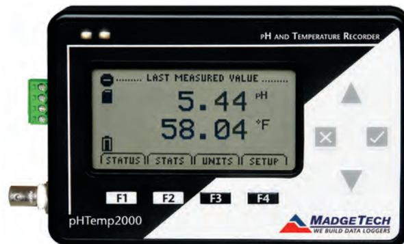
The storage medium is non-volatile solid state memory, providing maximum data security even if the battery becomes discharged. The device can be started and stopped directly from your computer.
