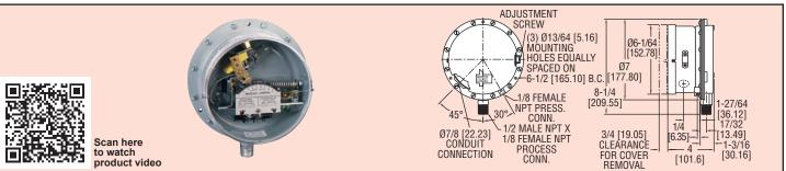
Large diaphragm sensitivity and time proven dependable design are combined in model PG differential pressure switches. Visible dial reduces "start up" time and helps prevent calibration errors. External adjustment allows set point change without removal of cover. Unit is listed by UL, FM and CSA.
