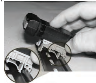
Figure 7. Snapping the Module to the DIN Rail
