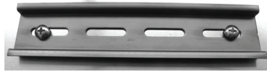
Figure 5. Mounting the DIN Rail with 2 #10 Pan Head Screws
